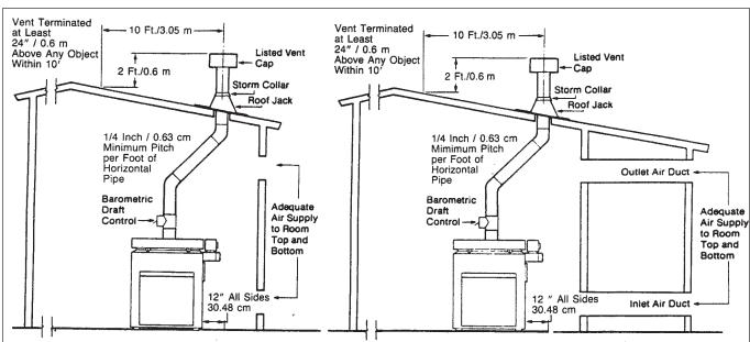
Figure 5. Combustion Air, Indoor Installation.
