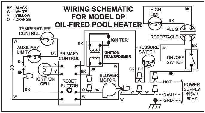
Figure 14. Wiring Diagram, 60 Hz Model.
