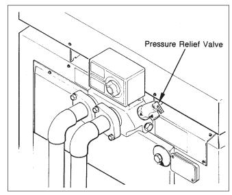
Figure 13. Pressure Relief Valve.
