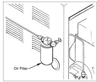
Figure 8. Oil Filter Installation.
