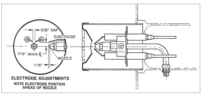
Figure 22. Electrode Adjustment.
