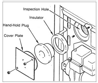
Figure 15. Inspection Hole Location.
