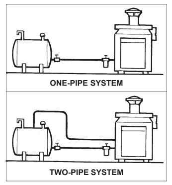
Figure 7. One-Pipe and Two-Pipe Systems.
