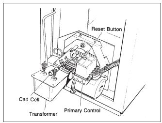
Figure 21. Cad Cell and Primary Control.
